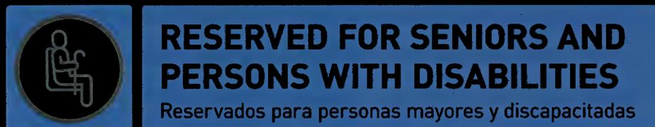
In addition to decals identifying the reserved seats a special seat covering has been developed that has the new pictogram woven into the fabric. The fabric will be produced in a color that contrasts with the other seats on buses and rail vehicles to distinguish the reserved seating and further discourage younger and fully ambulatory persons from sitting in the reserved seats.
