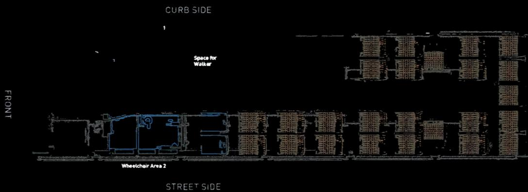
Revised layout with flip up seats in up position accommodating two (2) wheelchairs and one (1) walker.
