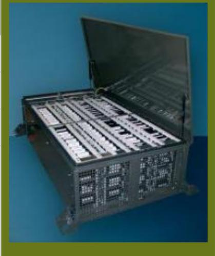
Typically one such box is installed per vehicle. Since the two traction inverters are connected on the high voltage side through the common High Speed Circuit Breaker (HSCB), one storage device can store the brake energy of both trucks.
