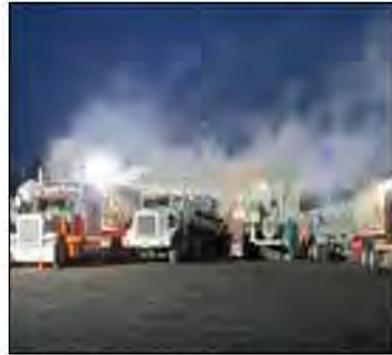
*Silica dust clouds from trucks loading into sand movers*
