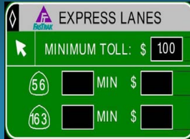
Typical Intermediate Access Point Entry Sign (from General Purpose Lane)
