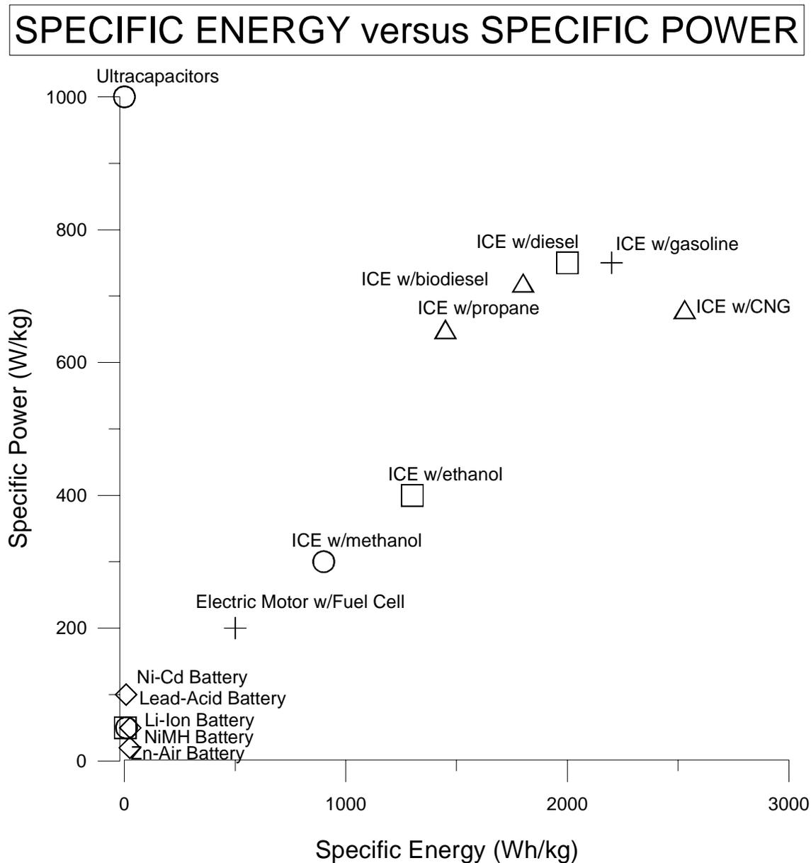
Figure 1. Power density and Energy density for various propulsion concepts
