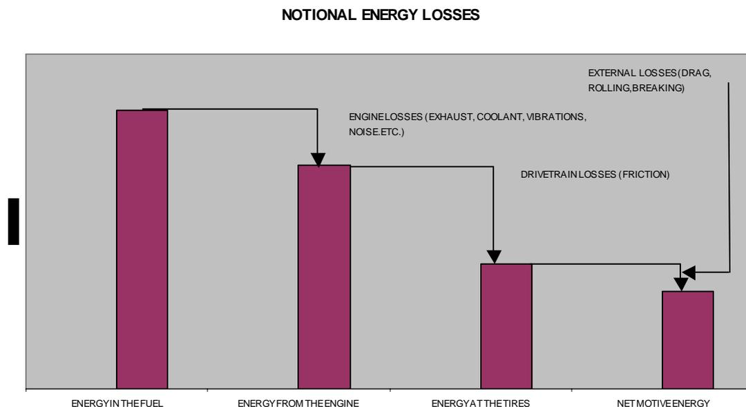
Figure 5- Energy Distribution Along the Systems in a Vehicle
