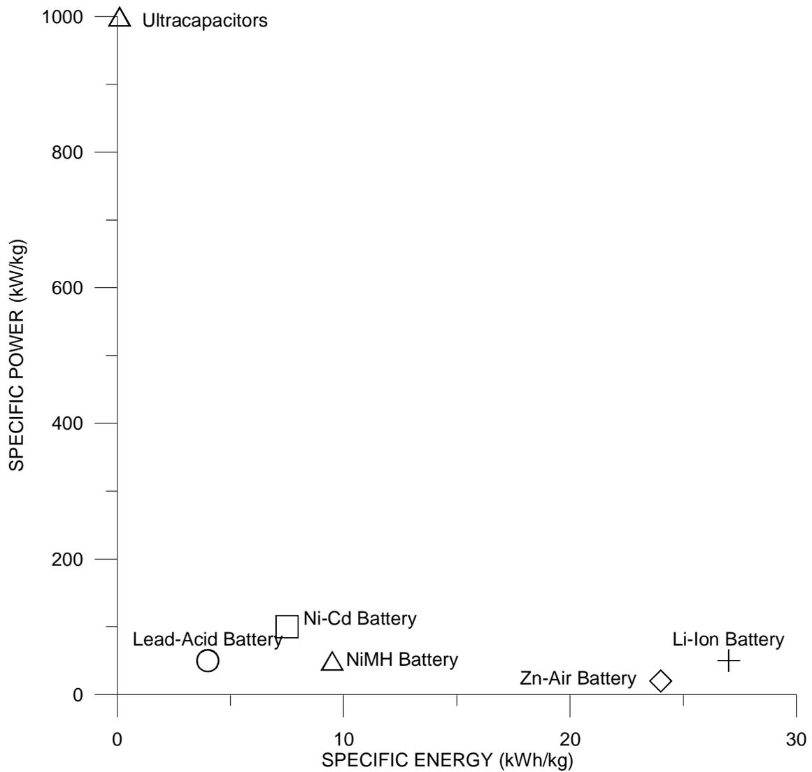
Figure 4. Specific Power vs. Specific Energy for Batteries and Ultracapacitors.
