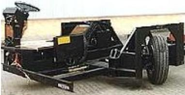
Figure 3- Common subassembly for ICE bus and trolleybus.
