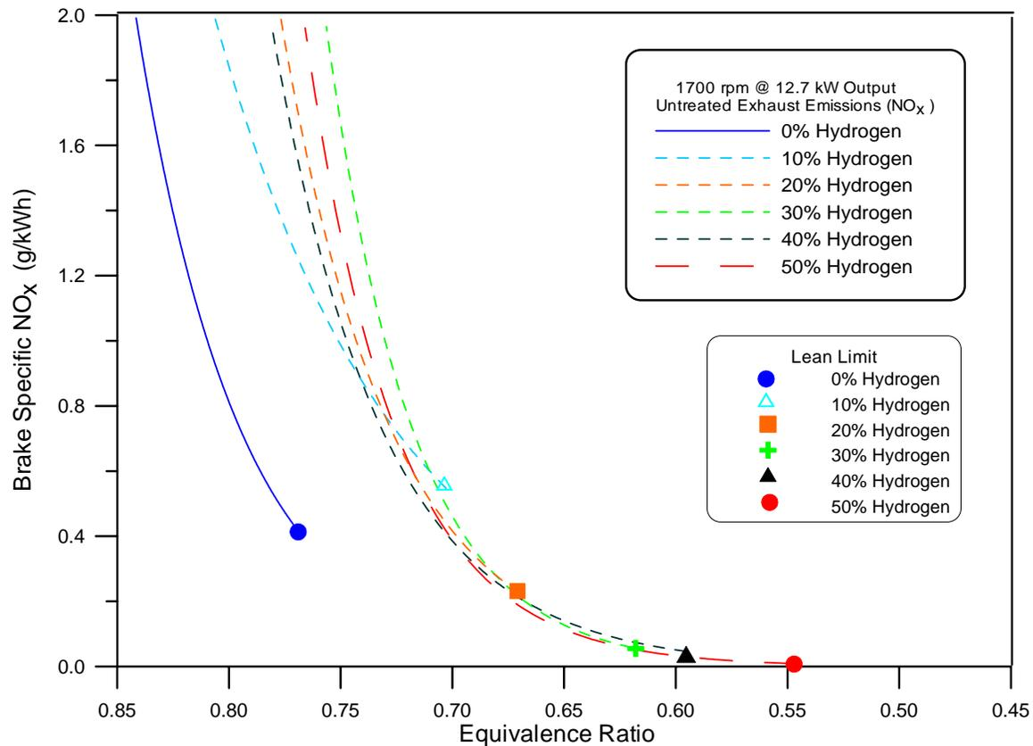
Figure 3- NO<sub>x</sub> emissions versus equivalence ratio (lean burn) for various hydrogen contents
