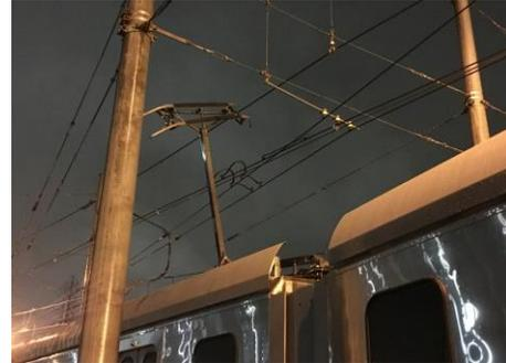
**Figure 16: Pantograph entanglement with OCS wires**
