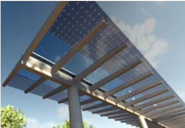
Figure 3-4 Rendered concept of a combination of bifacial solar panels and glass panels without a framed assembly on SWSD canopy.
