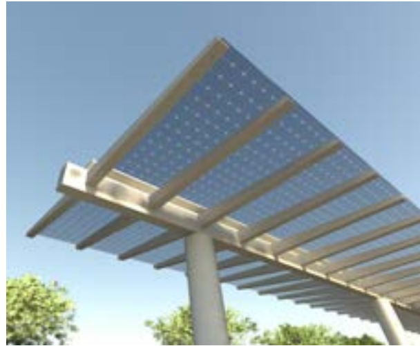
Figure 3-2 Rendered concept of continuous bifacial solar panels on Systemwide Station Design (SWSD) canopy.
