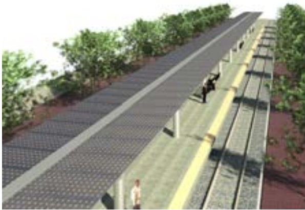
Figure 3-3 Rendered concept of continuous bifacial solar panels on SWSD center platform station with canopy running full length of platform to maximize energy production and shade on platform.
